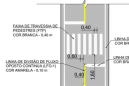
**DETALHE - LINHA SIMPLES CONTINUA - LFO-1 SEM ESCALA**
